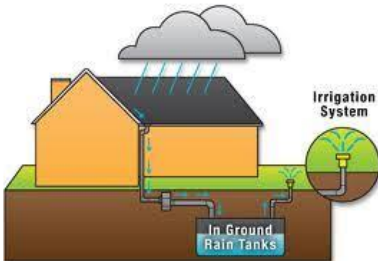
Example of a cistern that acts as a holding tank for irrigation water.
